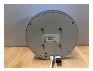
Load the content onto a standard USB Flash Memory (without folders and .trash files .....best with a Windows PC) and plug it into the micro USB socket with the enclosed USB adapter. Video resolution 1080x1080 pixels, video format .mp4, Codec H264, Bitrate approx. 10 Mbit/sec.
