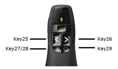
You can define custom commands to the keys, as described in <u>chapter 9.1 (Manual access via ftp client)</u>. The 4-5 Keys are Key25 to Key29.
